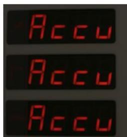
In case of a power failure “Accu” will appear on the control panel and the temperature indicators will switch off. Add-on modules such as air spa, light therapy etc. will automatically switch off.
